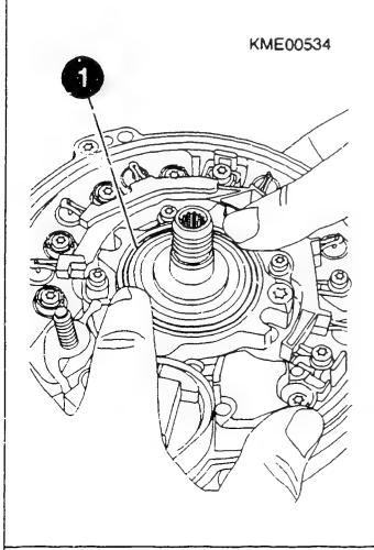
ASSEMBLING ALTERNATOR Fitting cap Mount new cap (1). ATTENTION: Position of O-ring (2) is not to be altered. Correct if necessary.
